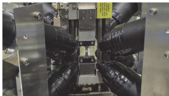
Fig. 1. A view of a small tensile tester installed at the BLIU beamline with a tensile test piece attached.
